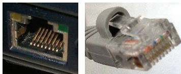
Ethernet Connector Left: on the computer Right: on the cable
